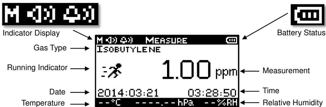
**Figure 3:** Annotated measure screen of the HVX501
