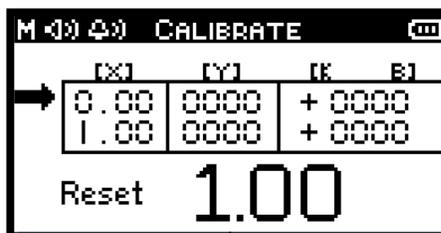
**Figure 8:** Calibrate Screen with Zero Measurement Complete
