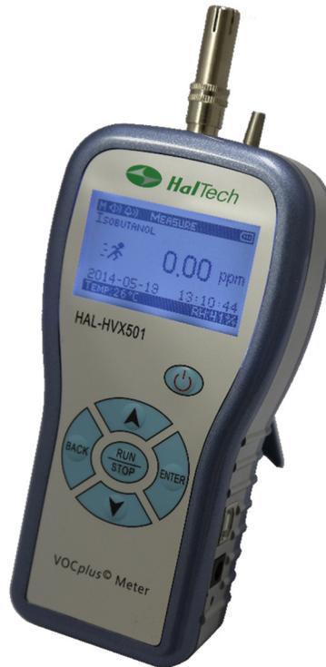
**Figure 1:** HAL-HVX501 Volatile Organic Compound (VOC) Meter
