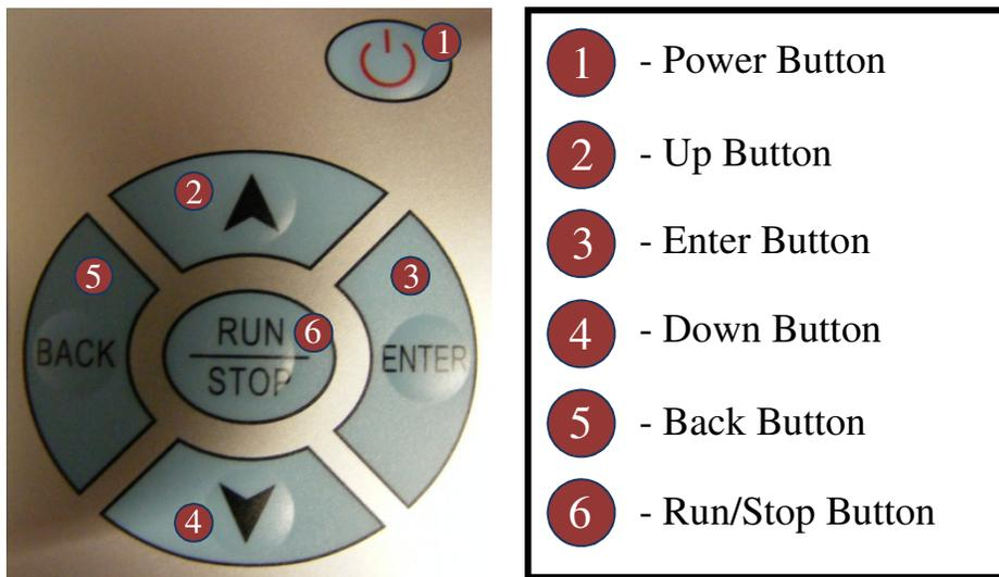
**Figure 2:** Close-up of the gas meter interface.
