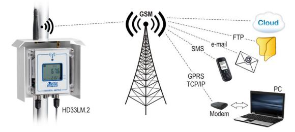
The data logger GSM functions can be remotely controlled by sending SMS messages.
